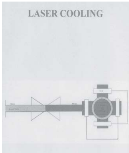
Figure - 5: Overall schematic of the cooling and trapping process of the atoms in an atomic beam. Atom are trapped first by a set of six mutually orthogonal laser beams (optical molasses) and subsequently trapped and cooled by magetic field
