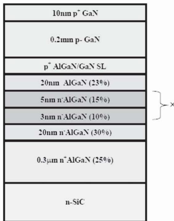
Figure - 4: Nano-Layer UV-LEDs Structure
